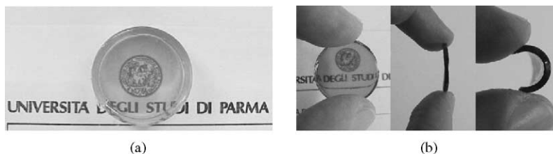
Fig. 1. View of (a) an aged hybrid monolith containing Siphen and TEOS in 1:2 ratio (fluoride catalysis) and (b) a flexible Siphen TEOS 1:2 monolith obtained in DMF with acid catalysis. The diameter of monoliths is about 2 cm.
